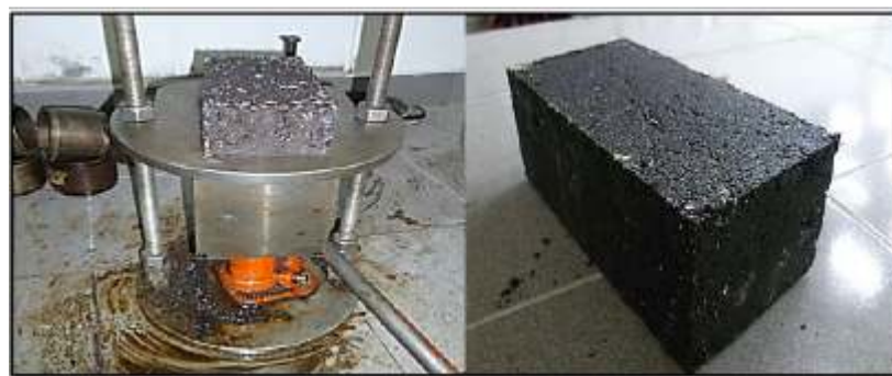
Fig. 4: Extruding of asphalt block from steel mold by a jack
