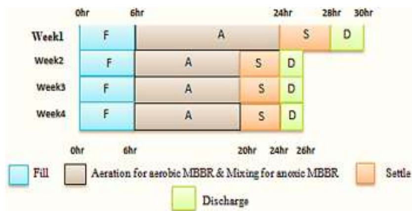
Fig. 2: Batch running cycle mode under start-up phase
