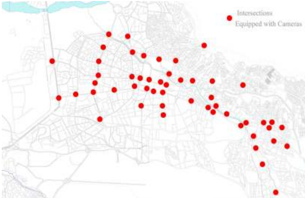
Fig. 3: Position of traffic control cameras in the network of passageways
