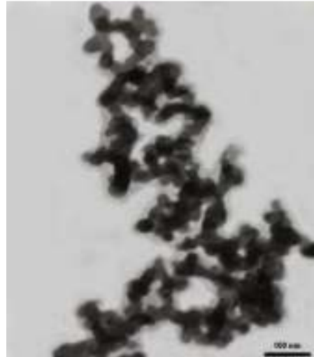
Fig. 1: TEM micrograph of synthesized super-paramagnetic iron oxide nano-particles
