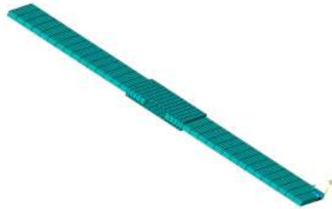
Fig. 5: Mesh model for FEA
