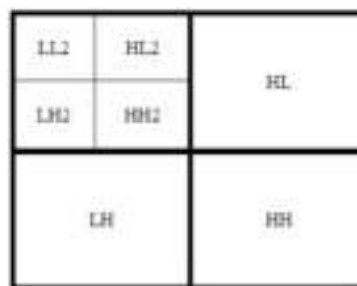
Fig. 1: A DWT decomposed image, its 4 bands (LL, HL, LH and HH) and second level sub-bands LL2, HL2, LH2 and HH2
