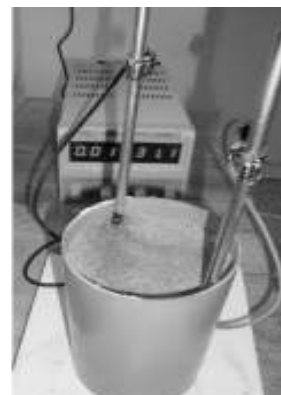
Fig. 2: Experimental set up for electroosmotic treatment of fine sand/resin mixes
