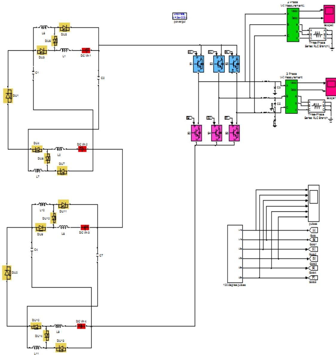
Fig. 3: Proposed modified embedded switched inductor Z-source inverter
