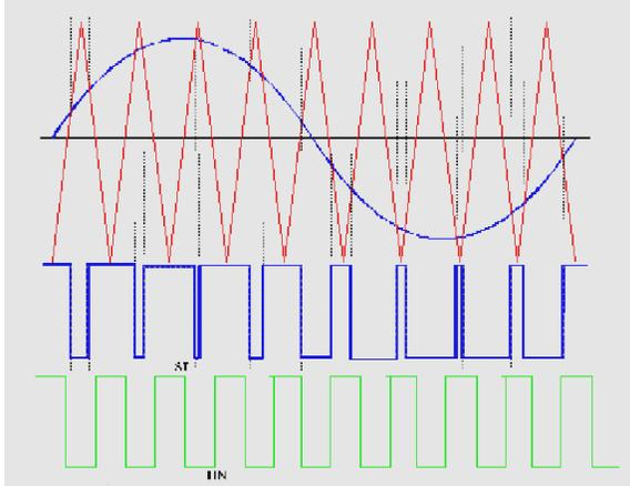
Fig. 5: Obtained PWM switching signals
