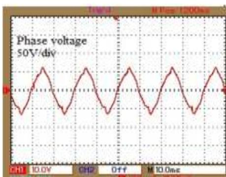
Fig. 13: Experimental phase voltage waveform, observed with filter
