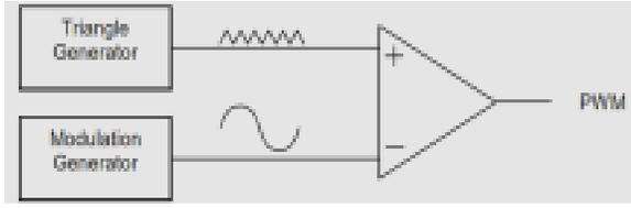
Fig. 4: PWM signal generating unit
