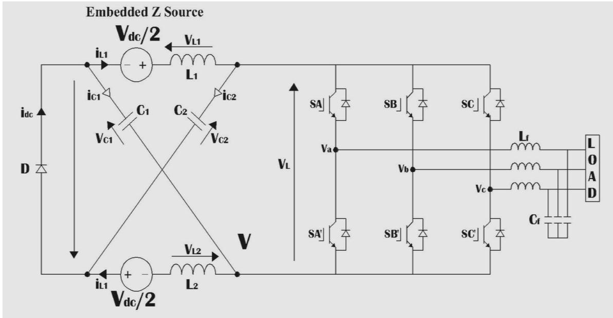
Fig. 1: Two level embedded Z source inverter
