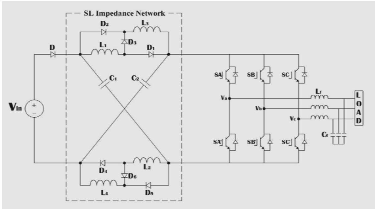
Fig. 2: Switched inductor Z source inverter
