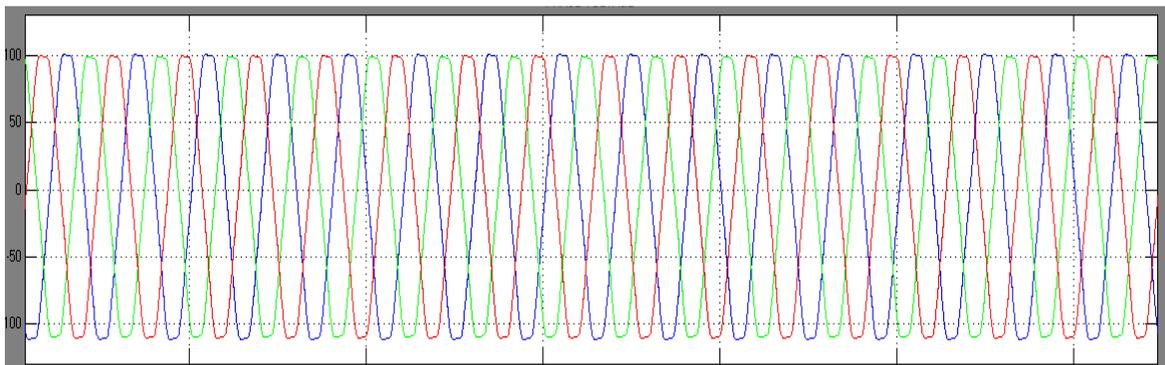
Fig. 6: Simulated output voltage waveforms of proposed inverter observed with LC filter (Scale: Y axis: 50 V/div)
