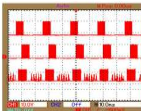
Fig. 15: Gate switching pulses observed across the inverter terminals
