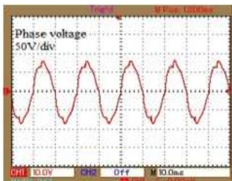
Fig. 12: Experimental phase voltage waveform, observed without filter
