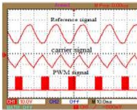
Fig. 16: Gate switching pulse observed for a single switch
