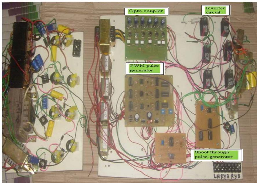
Fig. 11: Interior view of the proposed inverter
