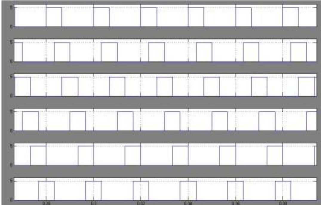
Fig. 7: Switching sequence of the proposed inverter ( $S_1$  to  $S_6$ )
