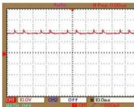
Fig. 17: Shoot through pulses observed for a single switch
