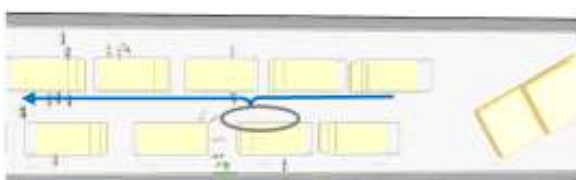
Fig. 18: Trajectory of the passenger escaping from the right front door of car C1 (scenario 1): the agent has to bypass the highlighted area afflicted by toxic smoke
