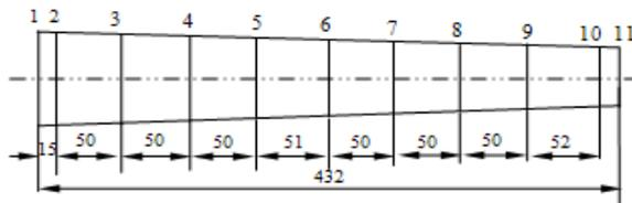
Fig. 6: Segments of twisted blade
