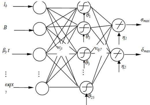
Fig. 10: BP model of blade
