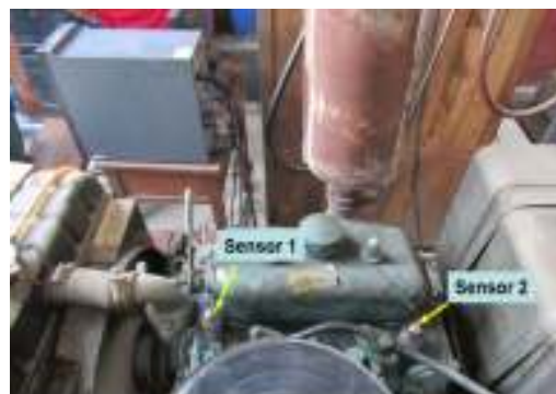
Fig. 2: The position of sensors on the diesel engine head
