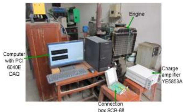
Fig. 1: Diesel engine fault diagnosis system, physical map
