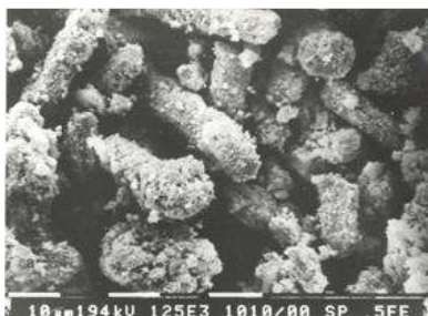
Fig. 4: Precipitated form of silver tungstate doped with iron tungstate, (0.83% FeWO 4 doped Ag 2 WO 4 )
