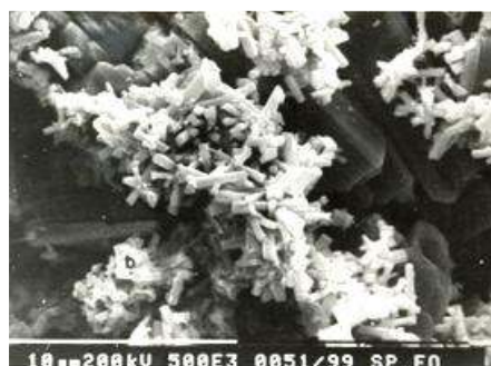
Fig. 3: Precipitated form of silver tungstate \text{Ag}_2\text{WO}_4 (x5000)
