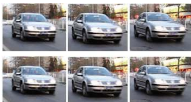
Fig. 6: Comparison with H.264 on 'car' video sequences. The first row shows the restored video sequences by proposed scheme and the second row shows the restored video sequences by H.264 with QP = 26
