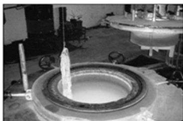
Fig. 3: Pit furnace used for the heat treatment of clad specimen
