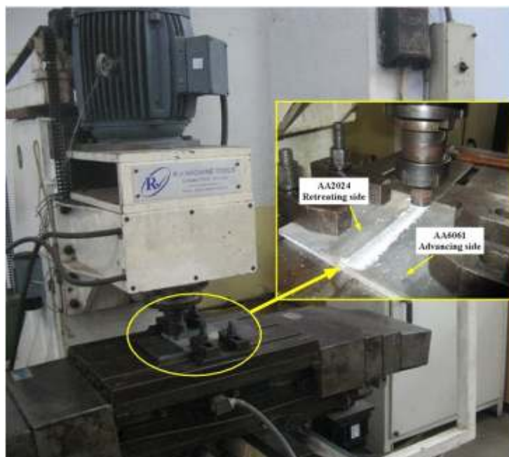
Fig. 1: FSW machine setup and position of aluminum alloys
