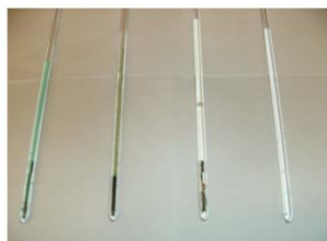
Fig. 19: Reactors with different metallic substances exposed to uncatalyzed esterification of lactic acid at 523 K. From left are reactors with stainless steel, inconel 625, tantalum sheet and reactor with no metallic substance
