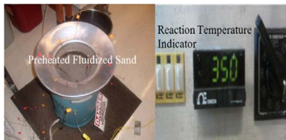
Fig. 1: Experimental setup of a batch reactor for esterification reaction
