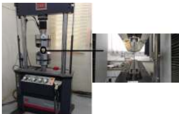
Fig. 5: Commercial pure copper sample during tensile test
