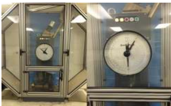
Fig. 6: Impact test machine using in this study
