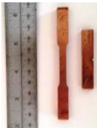
Fig. 4: Tensile and impact test specimens
