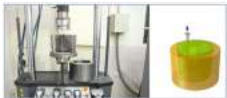
Fig. 2: ECAP die set-up used in this study
