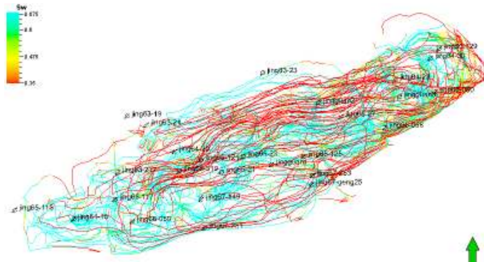
Fig. 17: Widespread of cold water flooding by frontsim in Jingguan 2 block (2013)
