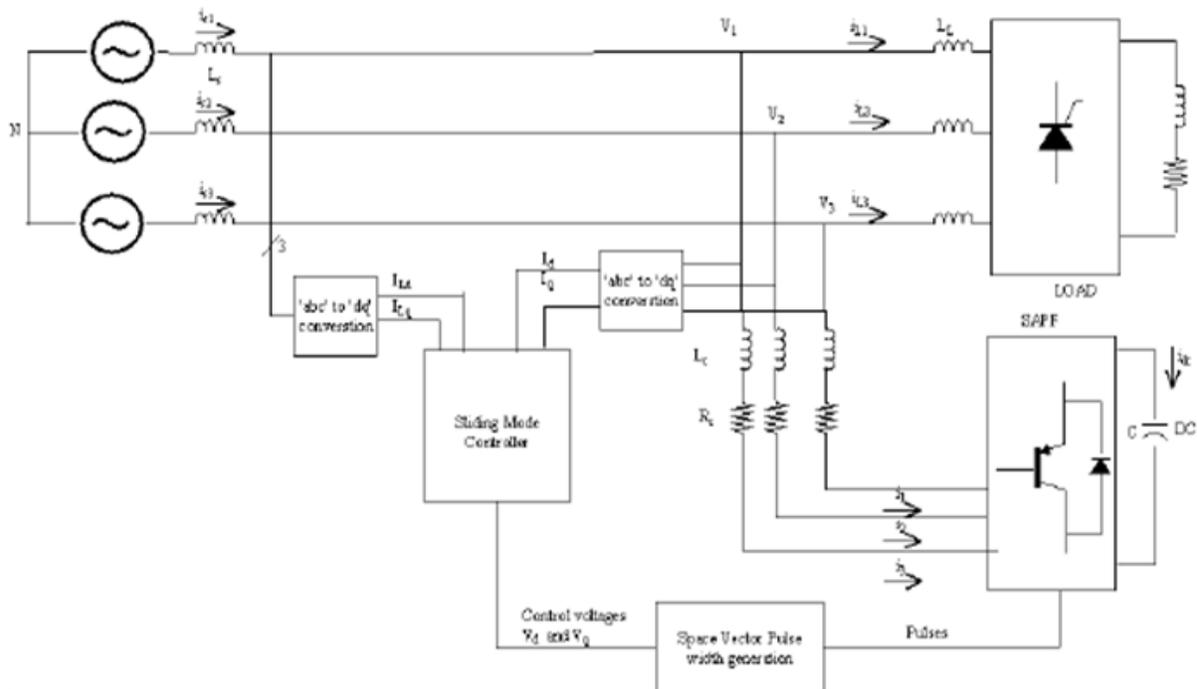
Fig. 2: Shunt active power filter with sliding mode control
