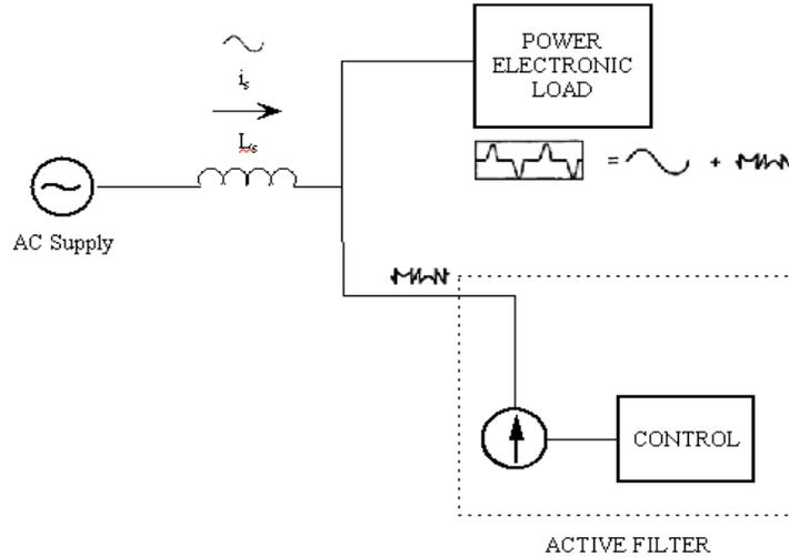
Fig. 1: Generalized shunt active power filter scheme
