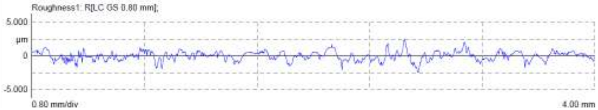
Fig. 23: Roughness plot after dry run test for composite bearing ( R_a = 0.5270 \mu\text{m} )
