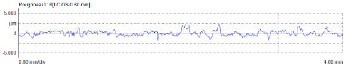
Fig. 22: Roughness plot before dry run test for composite bearing ( R_a = 0.4661 \mu\text{m} )
