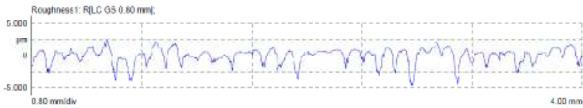
Fig. 24: Roughness plot before dry run test for gun metal bearing ( R_a = 0.8787 \mu\text{m} )
