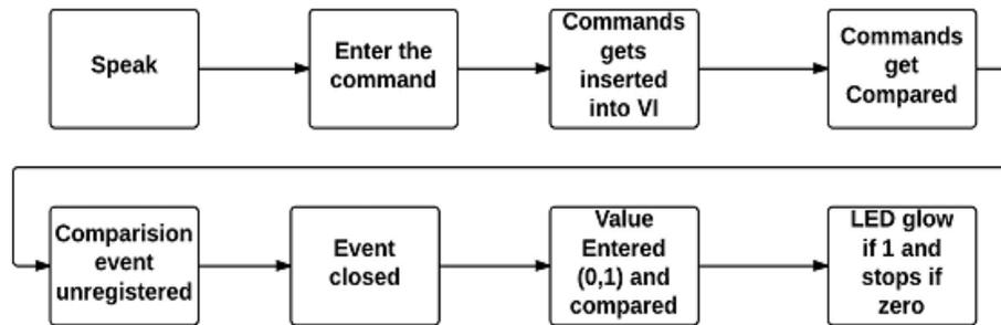
Fig. 2: Process by which voice integration with VI is done
