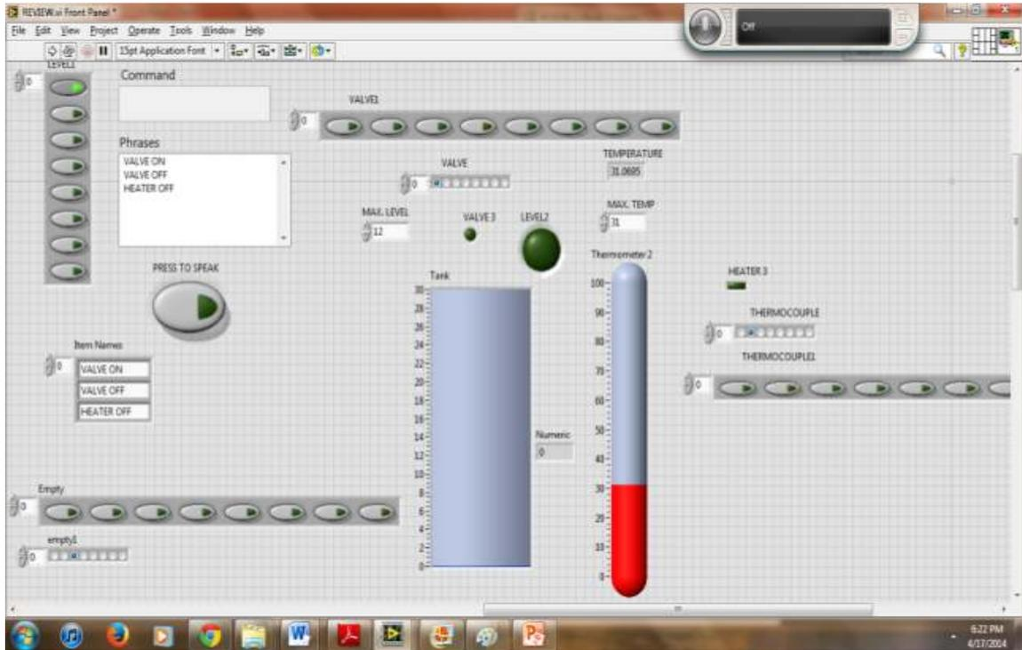
Fig. 5: Graphical user-interface of the geyser at the room temperature
