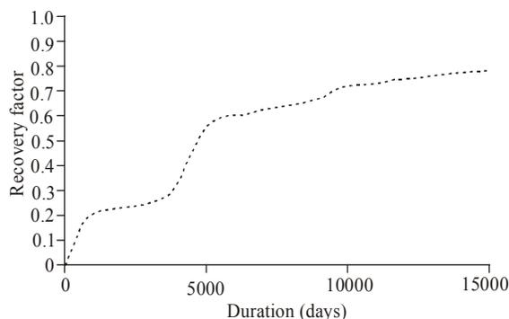
Fig. 4: Recovery factor during variable slug size injection
