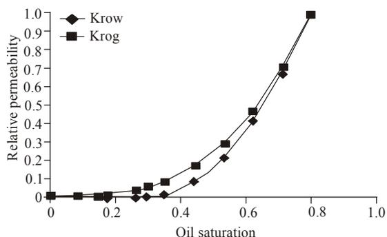
Fig. 3: Oil relative permeability curves versus oil saturation
