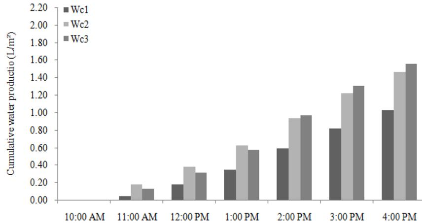
Fig. 12: Cumulative water production of solar stills S1, S2 and S3 on day 1 (April 4, 2013)
