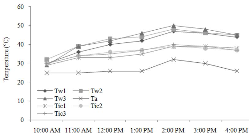
Fig. 7: Diurnal variations of temperatures of water, inner cover of solar stills and ambient air on day 1 (April 4, 2013)
