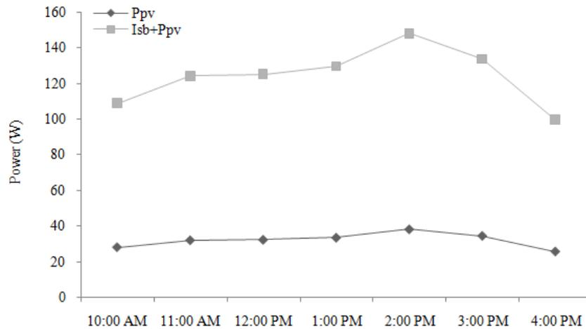
Fig. 6: Diurnal variation of the output power of 50 W photovoltaic module (P<sub>pv</sub>) and the cumulative power of I<sub>sb</sub> and P<sub>pv</sub> on day 1 (April 4, 2013)
