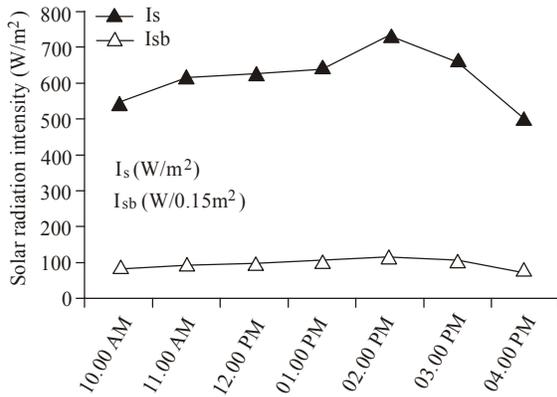
Fig. 4: Diurnal variation of solar radiation intensities per 1 m<sup>2</sup> (I<sub>s</sub>) and the solar radiation intensities on 0.15 m<sup>2</sup> basin area of each solar still (I<sub>sb</sub>) on day 1 (April 4, 2013)
