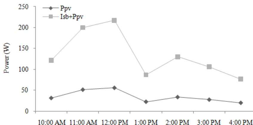
Fig. 8: Diurnal variation of the output power of 50 W photovoltaic module ( $P_{pv}$ ) and the cumulative power of  $I_{sb}$  and  $P_{pv}$  on day 2 (April 5, 2013)
