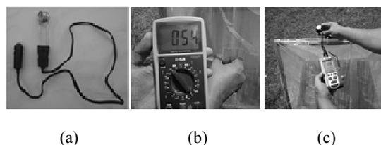
Fig. 3: Photographs of (a) 24 volt DC water heater, (b) digital multimeter (thermocouple), (c) solarimeter (SL200)
