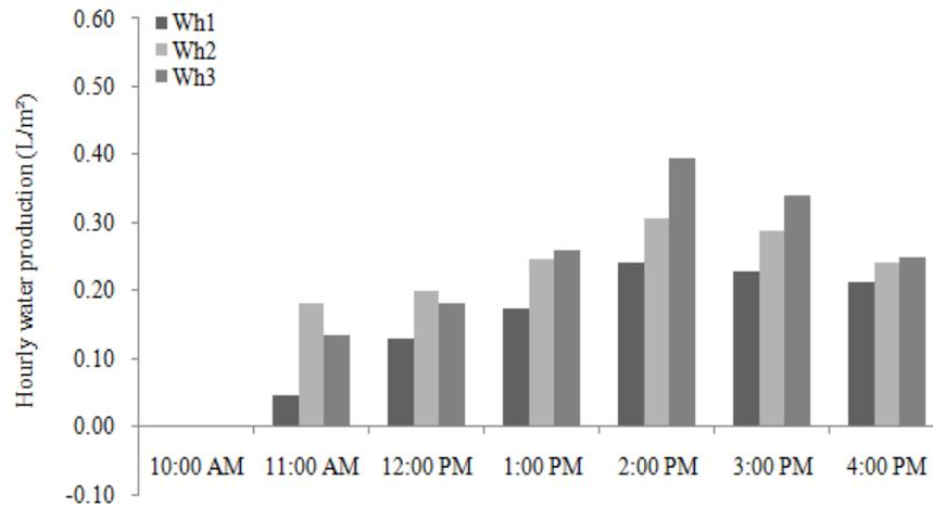
Fig. 10: Hourly water production of solar stills S1, S2 and S3 on day 1 (April 4, 2013)
