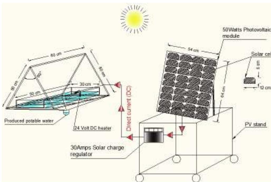
Fig. 1: Schematic diagram of solar still integrated with 50 watts photovoltaic module and 24 volt DC heater
