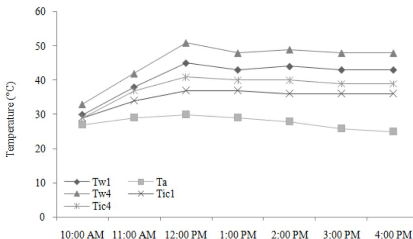
Fig. 9: Diurnal variations of temperatures of water, inner cover of solar stills and ambient air on day 2 (April 5, 2013)
