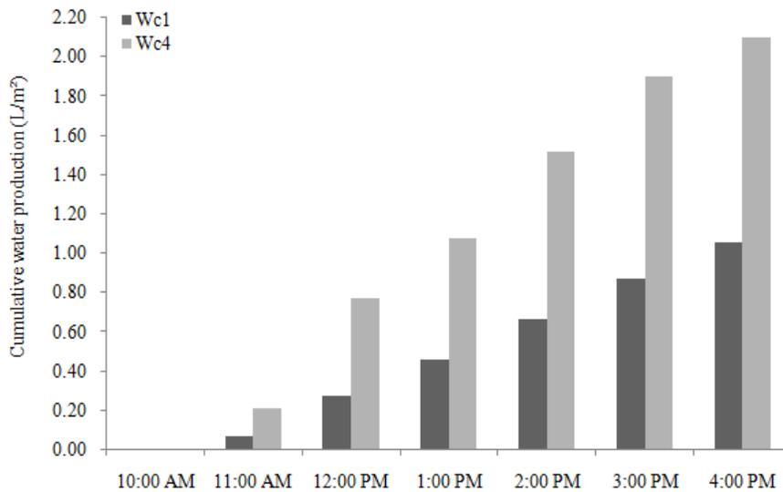
Fig. 13: Cumulative water production of solar stills S1 and S4 on day 2 (April 5, 2013)
