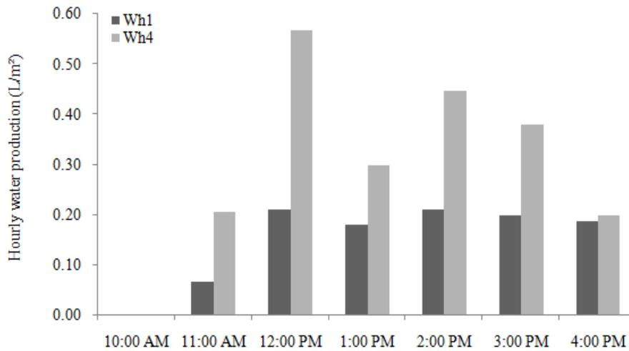
Fig. 11: Hourly water production of solar stills S1 and S4 on day 2 (April 5, 2013)
