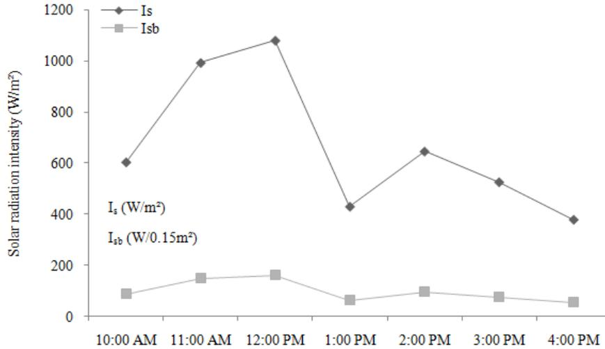
Fig. 5: Diurnal variation of solar radiation intensities per 1 m<sup>2</sup> (I<sub>s</sub>) and the solar radiation intensities on 0.15 m<sup>2</sup> basin area of each solar still (I<sub>sb</sub>) on day 2 (April 5, 2013)
