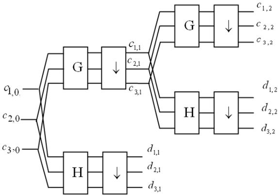
Fig. 1: Decomposition of multiwavelet transform
