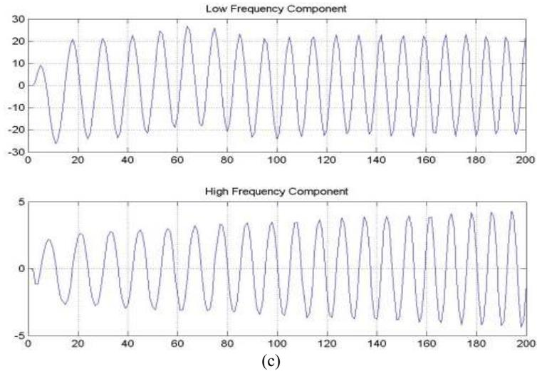
Fig. 5: Low and high frequency components of stator current for healthy induction motor; (Scale factor for x-axis of low frequency component in Fig. 5. a – c is 2)
