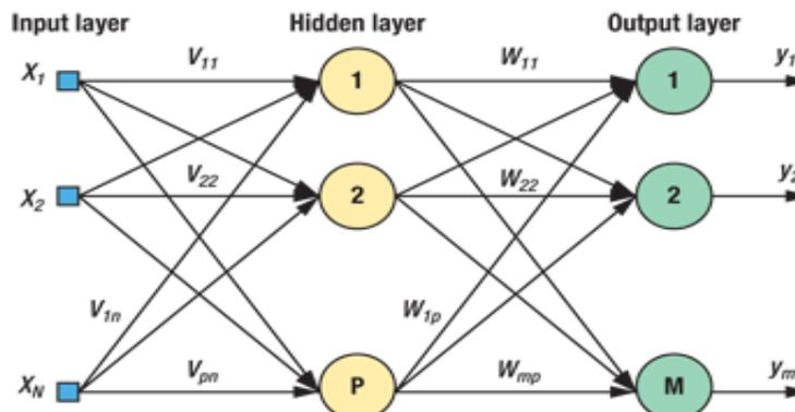
Fig. 2: Structure of neural network
