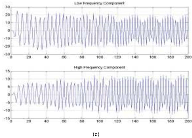
Fig. 6: Low and high frequency components of stator current for faulty induction motor; (Scale factor for x-axis of low frequency component in Fig. 5. a – c is 2)
