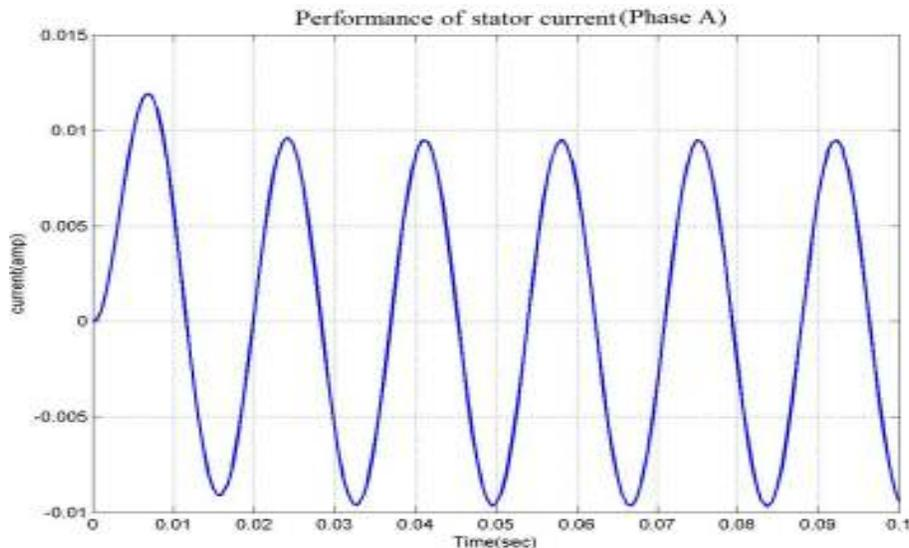
Fig. 3: Stator current for healthy induction motor
