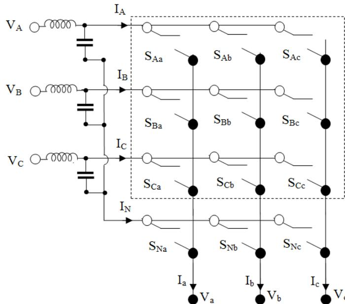
Fig. 1: Topology of the direct three-level matrix converter
