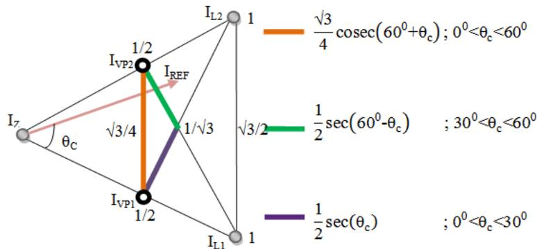
Fig. 5: Equations of lines used for identifying regions in the FTC
