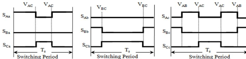
Fig. 10: Commutation events of the CMC in a switching period for voltage sector 1 and current sector 1
