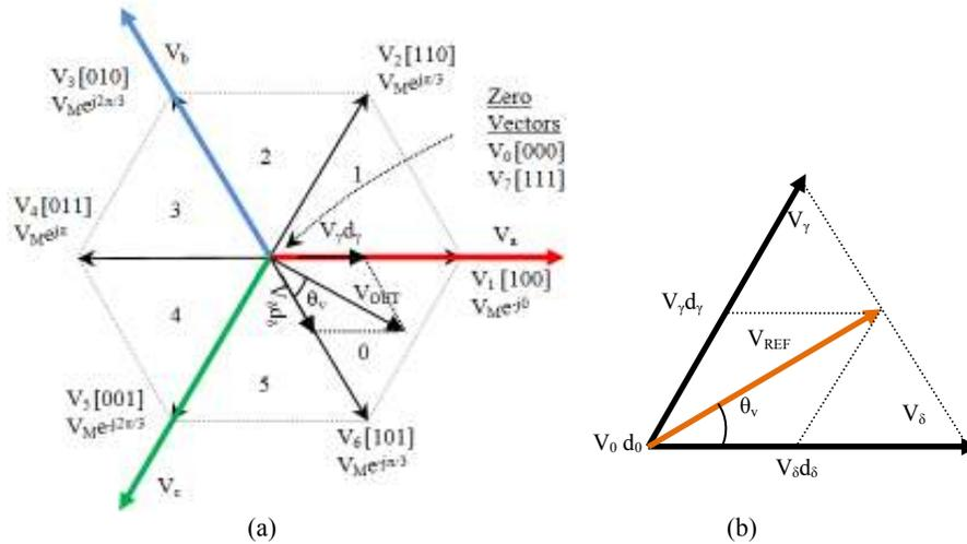
Fig. 7: (a) Space vectors of the FI and (b) sector and duty cycle allocation
