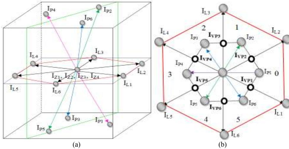
Fig. 3: (a) Space vectors of the FTC (b) space vectors and virtual vectors of the FTC
