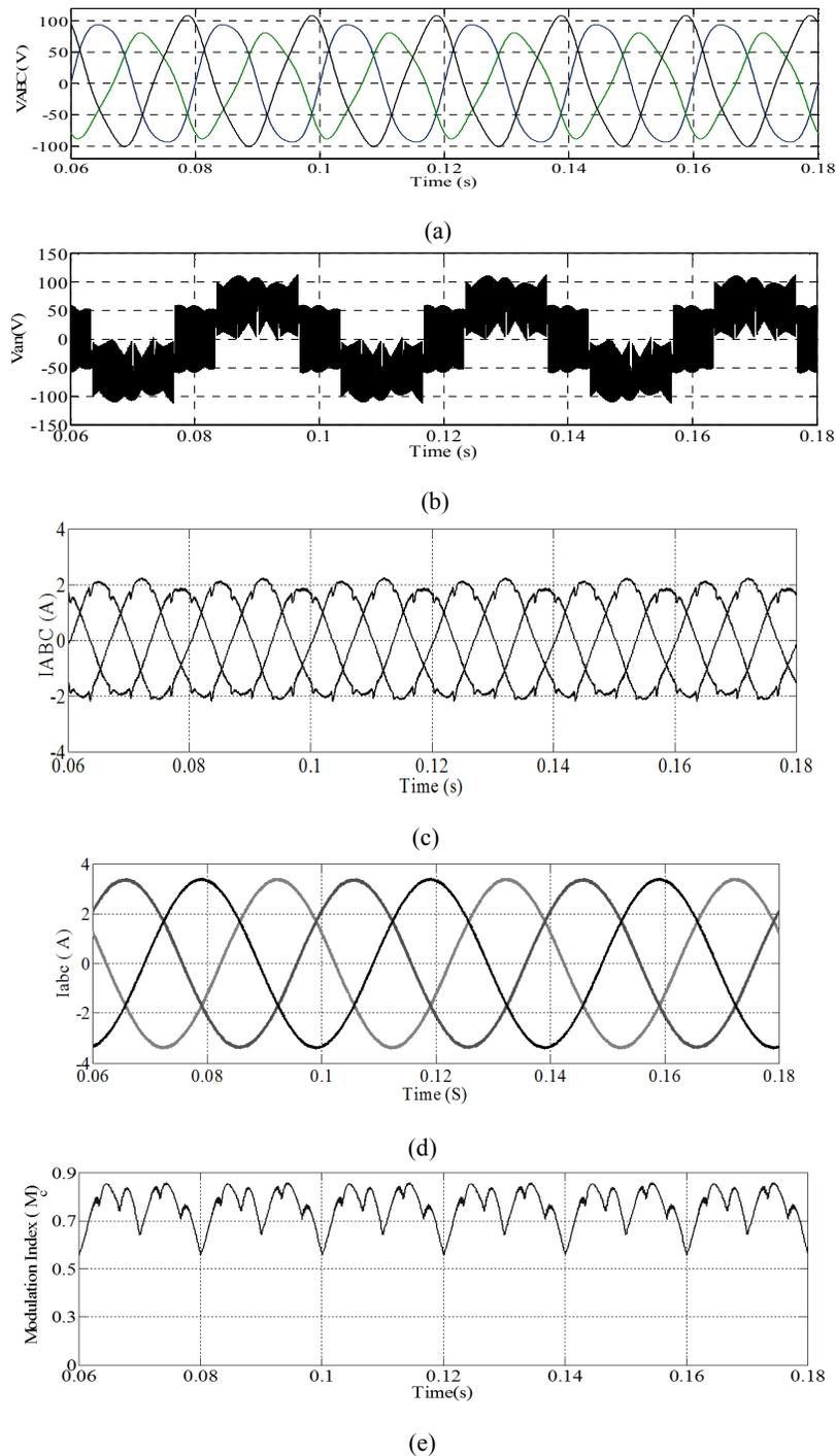
Fig.12: Performance of the DTMC with an unbalanced supply (a) output phase voltage, (b) output line voltage, (c) input phase current, (d) output phase current, (e) modulation index
