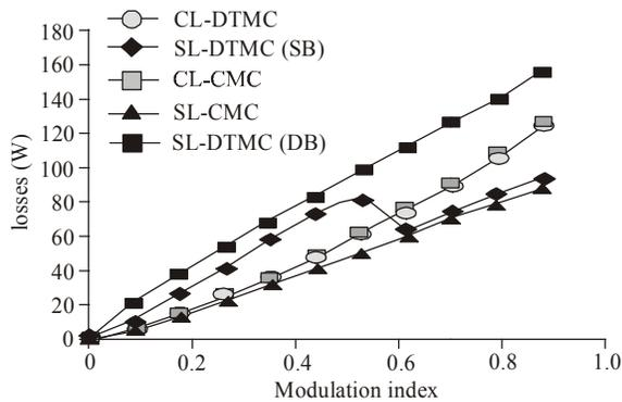
Fig. 15: Conduction and switching losses for the DTMC and the CMC for different values of MI
