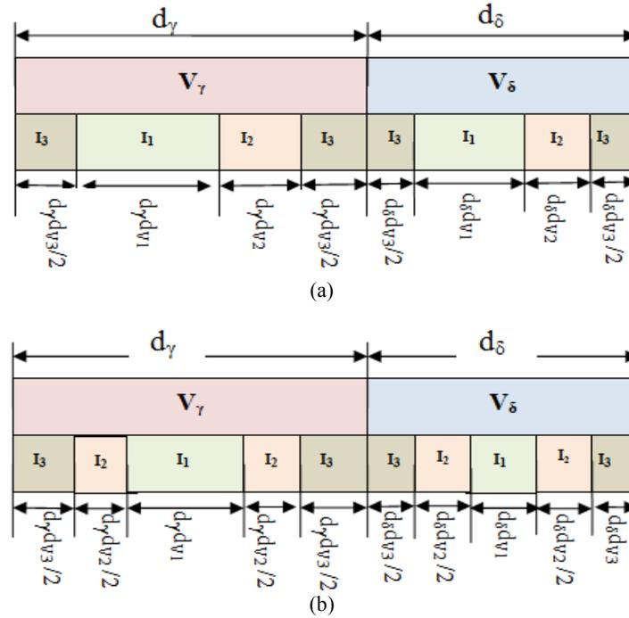
Fig. 8: (a) Switching pattern of the DTMC for the regions  $R_1$  and  $R_2$  (b) switching pattern of the DTMC for the regions  $R_3$ ,  $R_4$  and  $R_5$
