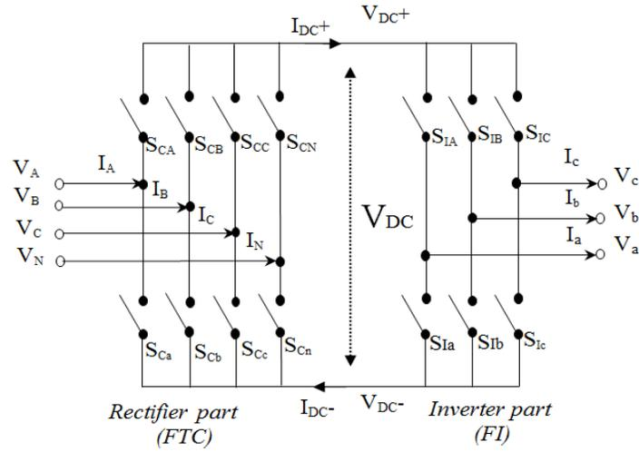
Fig. 2: Topology of the indirect three-level matrix converter
