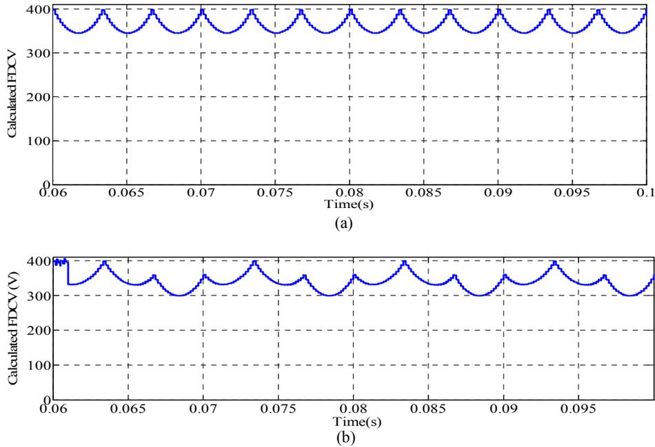
Fig. 9: (a) Calculated FDCV with a balanced input voltage (b) calculated FDCB voltage with an unbalanced input voltage
