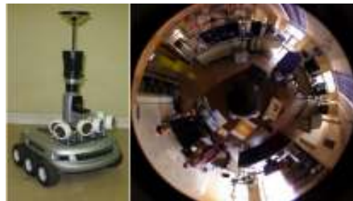
Fig. 1: An omnidirectional sensor mounted on mobile robot and the obtained omnidirectional image
