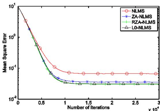
Fig. 13: MSE performance comparison for NLMS-based algorithms when the measured CIR is sparse at SNR of 10 dB
