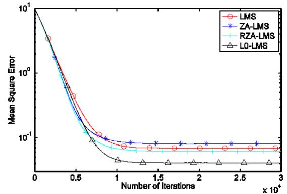
Fig. 4: MSE performance comparison for LMS-based algorithms when the measured CIR is dense at SNR of 10 dB
