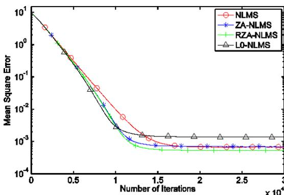
Fig. 15: MSE performance comparison for NLMS-based algorithms when the measured CIR is sparse at SNR of 30 dB
