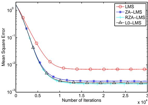
Fig. 8: MSE performance comparison for LMS-based algorithms when the measured CIR is sparse at SNR of 20 dB
