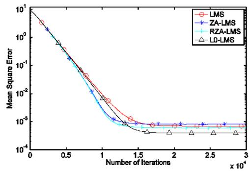
Fig. 6: MSE performance comparison for LMS-based algorithms when the measured CIR is dense at SNR of 30 dB
