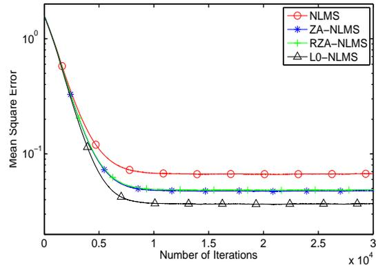
Fig. 10: MSE performance comparison for NLMS-based algorithms when the measured CIR is dense at SNR of 10 dB
