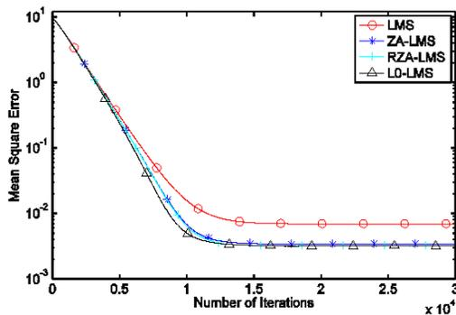
Fig. 5: MSE performance comparison for LMS-based algorithms when the measured CIR is dense at SNR of 20 dB
