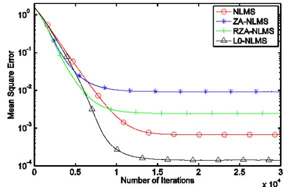
Fig. 12: MSE performance comparison for NLMS-based algorithms when the measured CIR is dense at SNR of 30 dB
