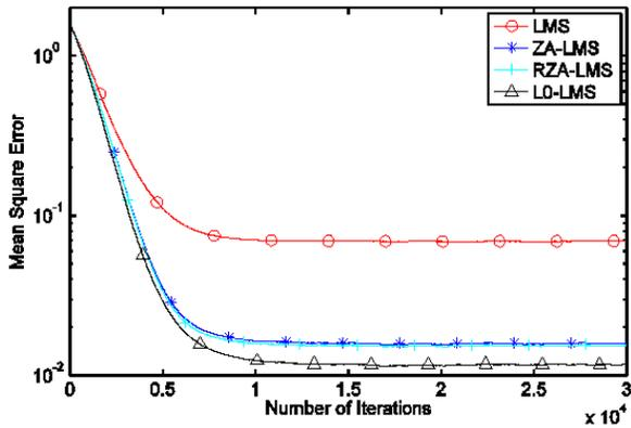
Fig. 7: MSE performance comparison for LMS-based algorithms when the measured CIR is sparse at SNR of 10 dB
