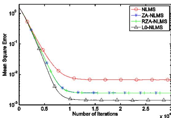
Fig. 14: MSE performance comparison for NLMS-based algorithms when the measured CIR is sparse at SNR of 20 dB
