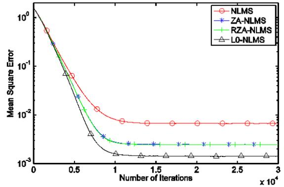
Fig. 11: MSE performance comparison for NLMS-based algorithms when the measured CIR is dense at SNR of 20 dB
