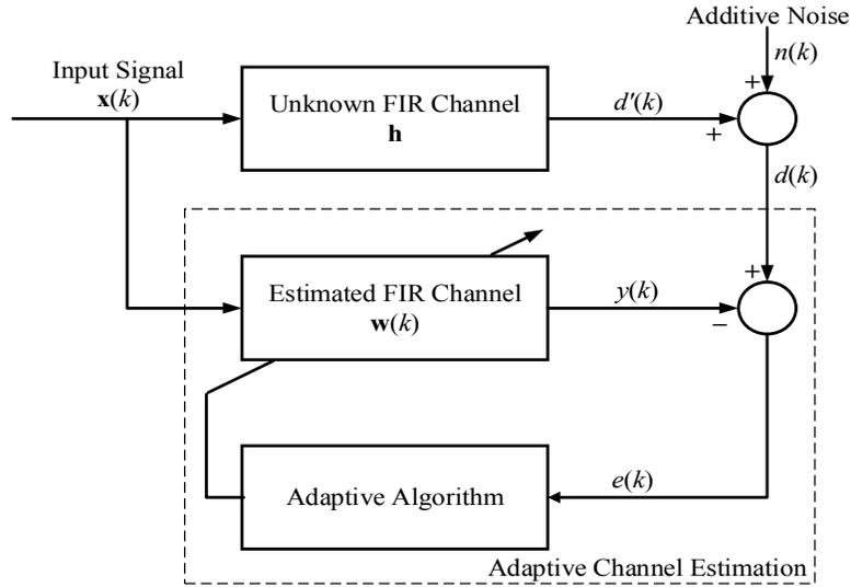
Fig. 1: A typical system identification block diagram
