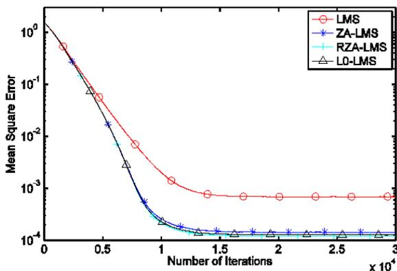
Fig. 9: MSE performance comparison for LMS-based algorithms when the measured CIR is sparse at SNR of 30 dB
