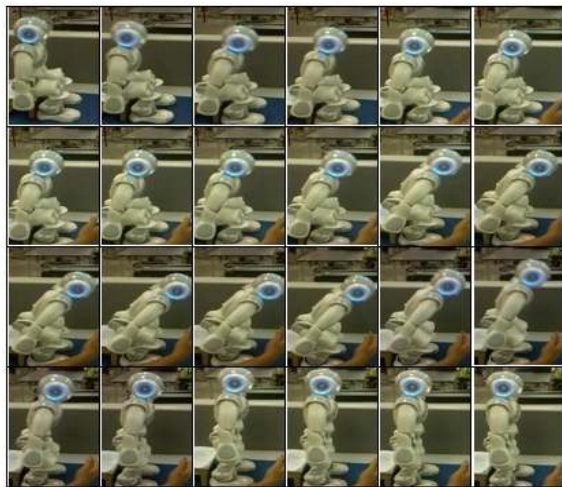
Fig. 13: Motion of the robot when G1 = 3000 , G2 = 1000 and G3 = 2500
