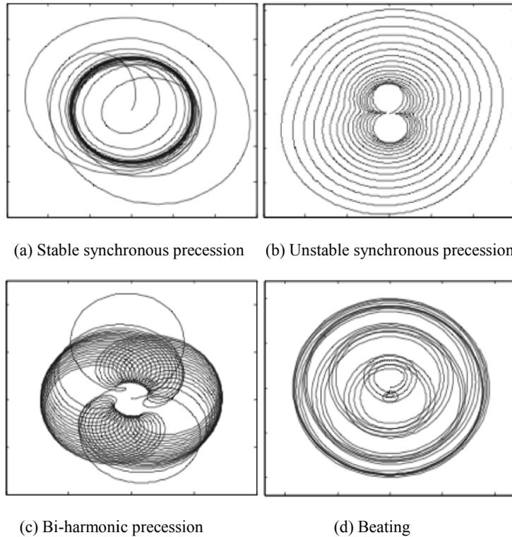
Fig. 5: Types of the rotor's oscillatory motion in the compliant support
