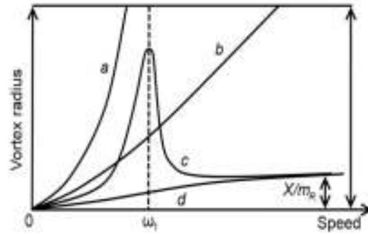
Fig. 3: The influence of the deformation on parametric resonance
