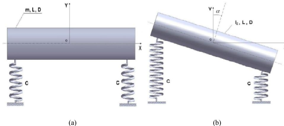
Fig. 1: The first (a) and the second (b) oscillation modes of the shaft
