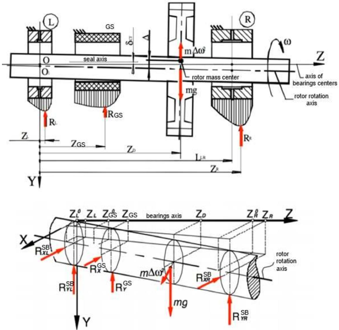
Fig. 2: Calculation scheme and the system of forces acting on the shaft, rotating with angular velocity  $\omega$ , having eccentricity  $\Delta$
