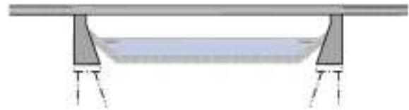
Fig. 3: Abutment (joint less) bridge
