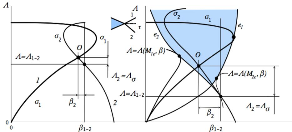
Fig. 4: Region of existence of the solution with two outgoing compression shocks at the given angle of interaction of flows  $\beta_{1-2}$  and relation of pressures  $\Lambda_{1-2}$
