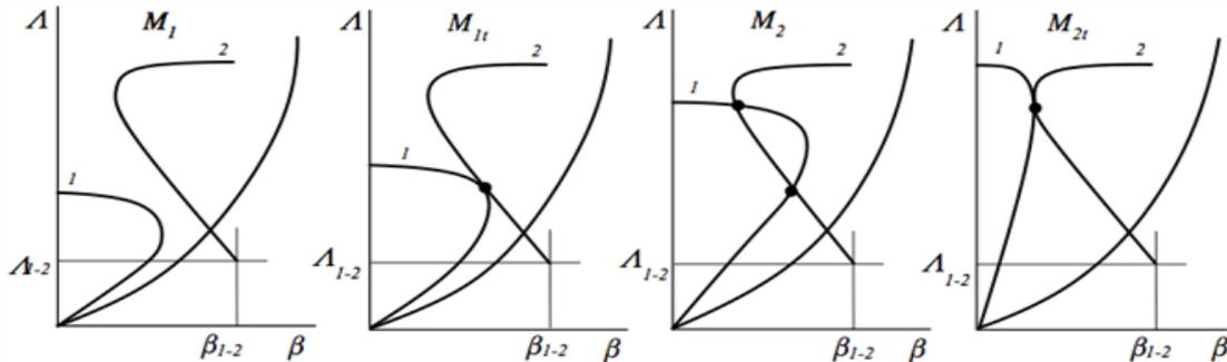
Fig. 5: Picture of solution on the polar plane at different mach numbers  $M_1 < M_{1t} < M_2 < M_{2t}$
