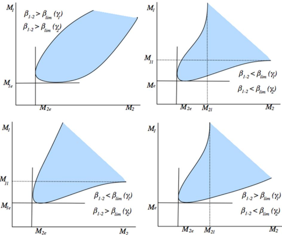
Fig. 6: Regions of solution existence for the problem of breakdown of an arbitrary discontinuity with formation of two outgoing compression shocks
