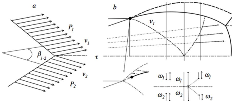
Fig. 2: Examples of streams with outgoing depression waves
