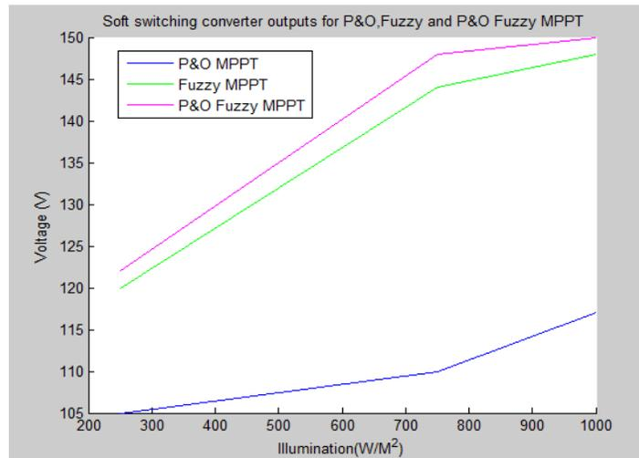
Fig. 14: Soft switching converter outputs for various algorithm
