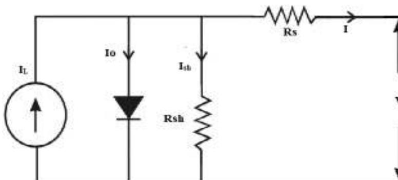
Fig. 2: Equivalent circuit of PV solar cell
