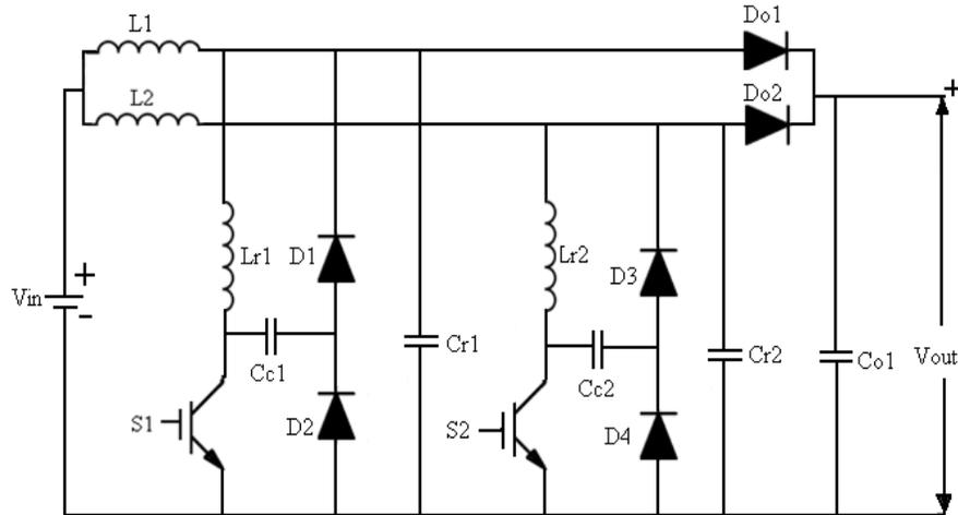
Fig. 6: Interleaved soft switching (resonant) converter
