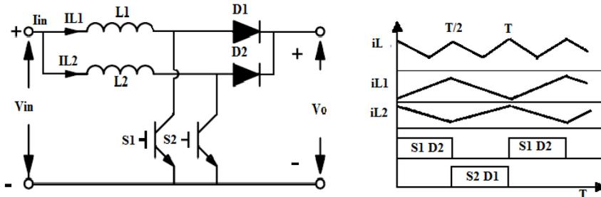
Fig. 5: Circuit diagram and wave forms of interleaved converters
