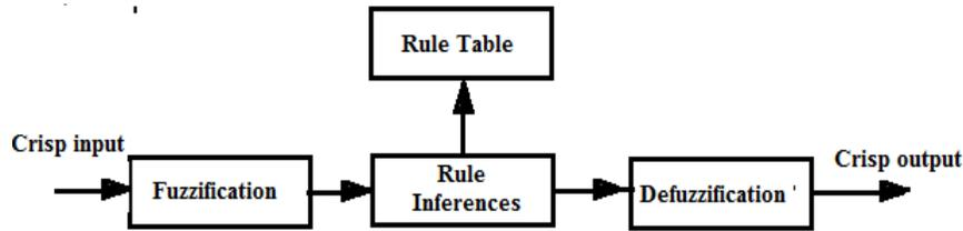
Fig. 9: Block diagram of FLC
