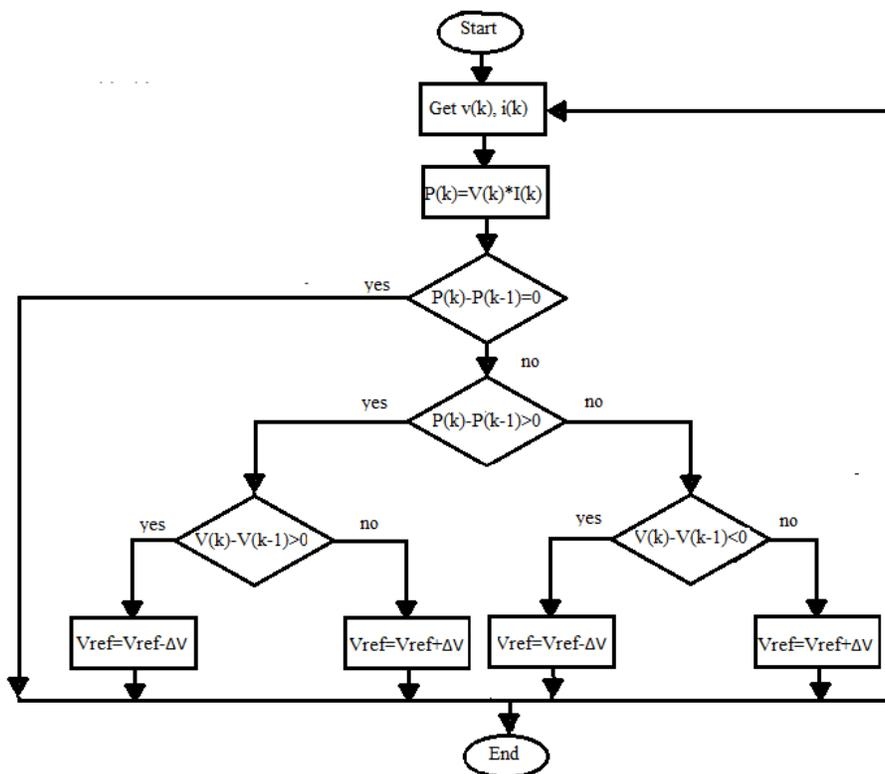
Fig. 7: Flow chart for P&O MPPT technique
