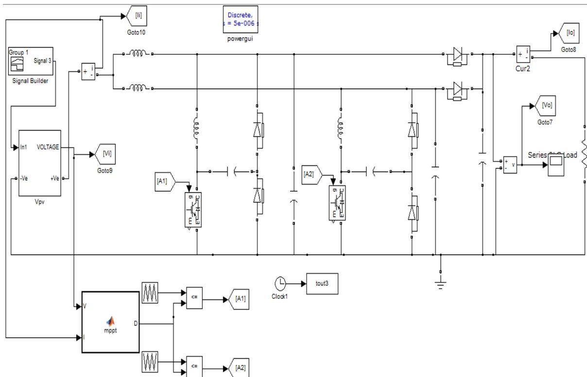
Fig. 11: Simulation of soft switching converter using MPPT
