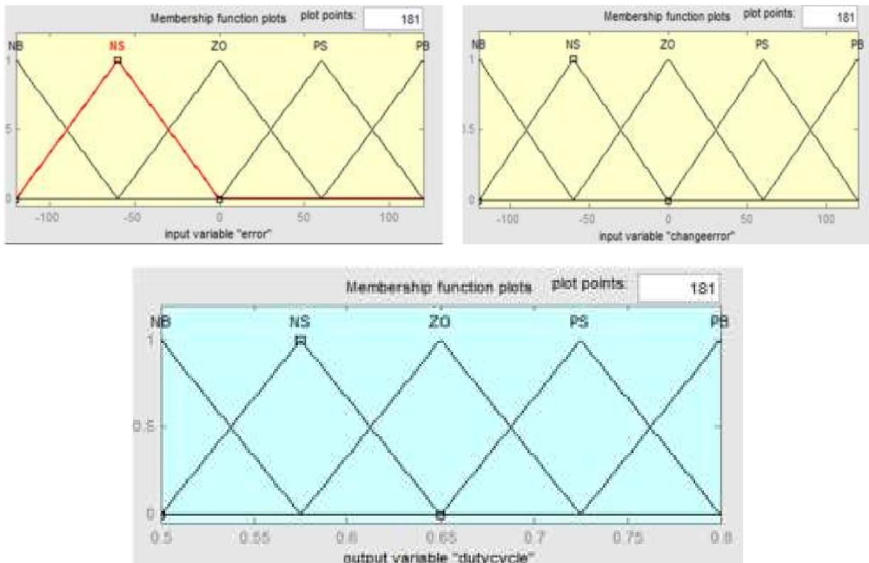
Fig. 10: Fuzzy logic membership functions for input and output variables
