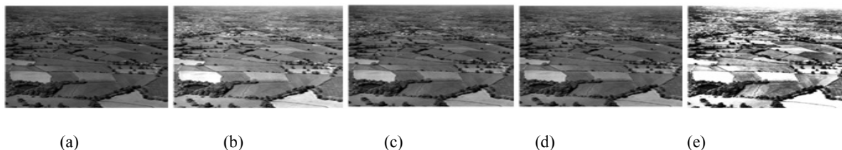
Fig. 14: (a): Original low contrast image; (b): Equalized image by the linear contrast stretching technique; (c): Equalized image by the GHE; (d): Equalized image by using Gamma correction technique; (e): Equalized image by the proposed methodology using SVD-DCT technique
