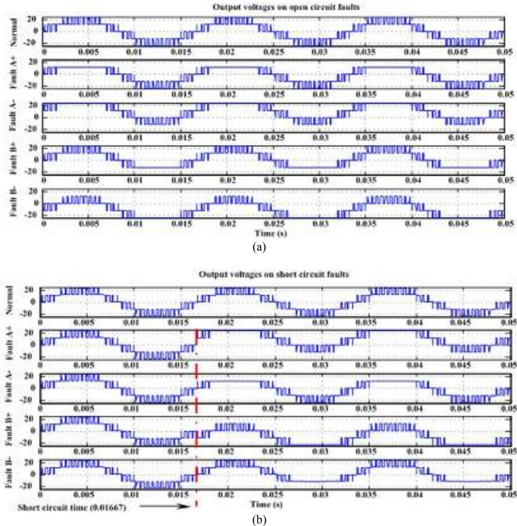
Fig. 5: Simulation of output voltages signals; (a): open circuit faults; (b): short circuit faults showing fault features at S, S, S and S of H-bridge 2 with modulation index = 0.8 out of 1.0
