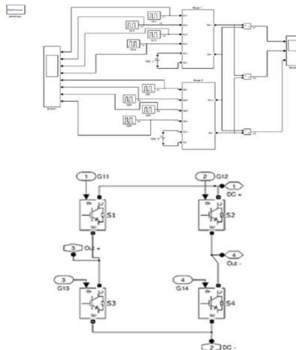
Fig. 9: (a): Single stage of an MLI; (b): Simulink model of a 5-level cascaded MLI
