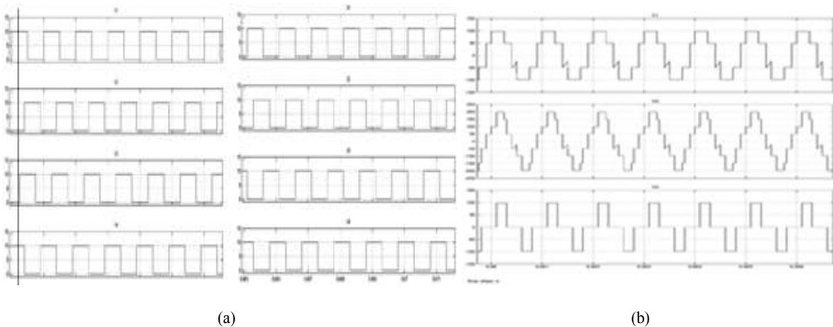
Fig. 12: Triggering pulses and output waveforms when the Switch S<sub>13</sub> is triggered 0.25 ms early
