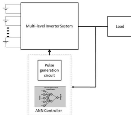
Fig. 8: General block diagram of an ANN controller based fault diagnostic system
