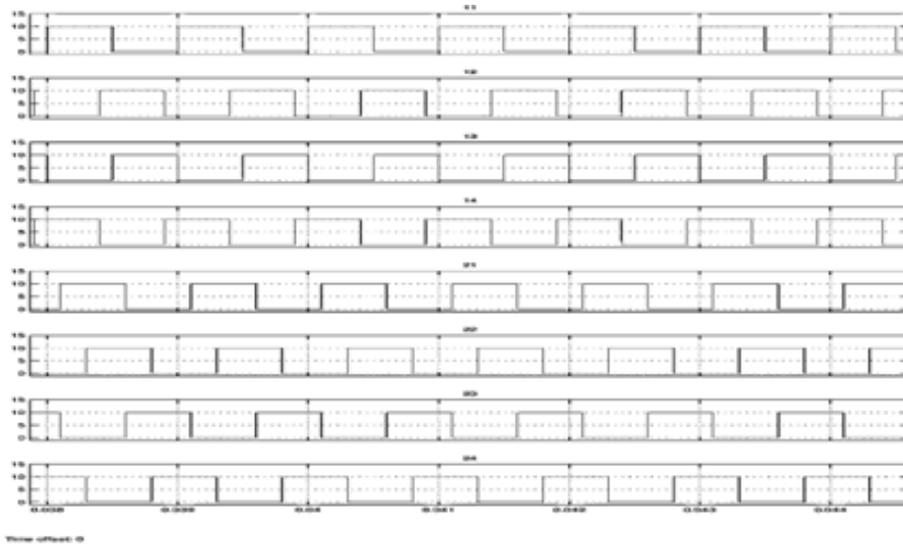
Fig. 10: Firingpulses to the healthy MLI
