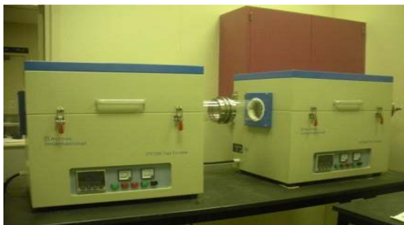
Fig. 2: Two stage reduction process based on the two STF1200-tube furnaces
