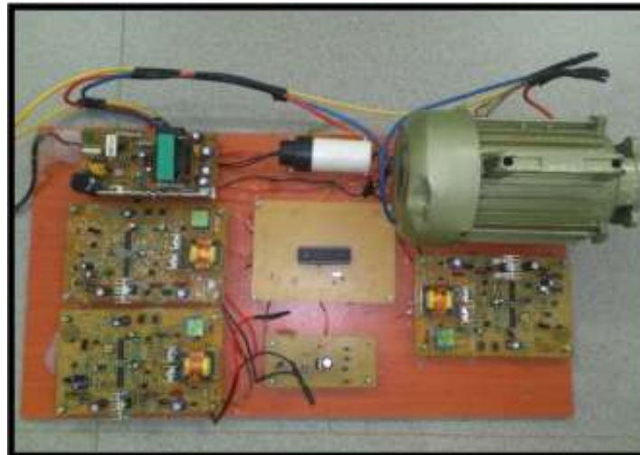
Fig. 9: Experimental setup for Dc-Dc converter for load application
