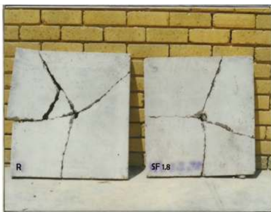
(A) Precast concrete slab reinforced with 1.8% by volume of sisal fiber
