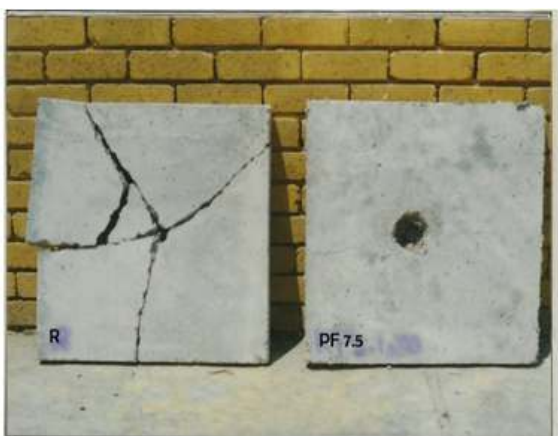
(B) Precast concrete slab reinforced with 7.5% by volume of palm fiber
