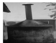
Fig. 2: The ferrocement furnace (Habeeb and Mahmud, 2010)
