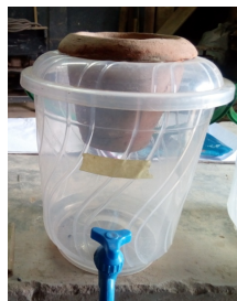
Fig. 19: Filtration of composition C 3 80 in a container
