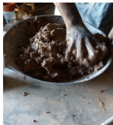
Fig. 8: Hand mixing of weighed materials
