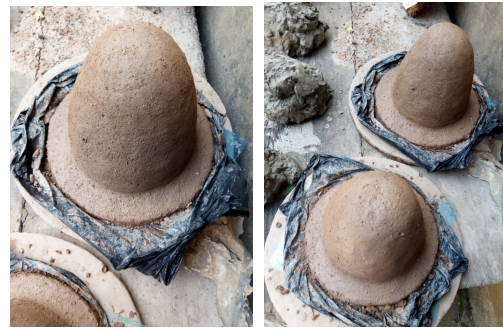
Fig. 11: Samples of pressed clay filters
