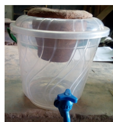
Fig. 18: Filtration of composition C 2 75 in a container
