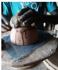
Fig. 9: Raw mold being used for pressing
