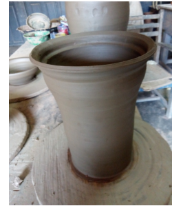
Fig. 12: Sample of smooth pressed clay filter ready for drying
