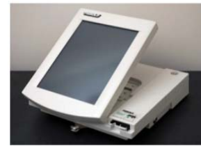
Fig. 3: The diebold AccuVote-TS, a touch screen based EVM (Ariel et al., 2006)
