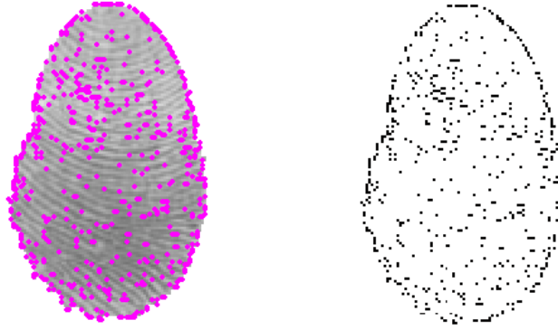
Fig. 6: Detection and extraction to corner points based on the algorithm of gray level jump
